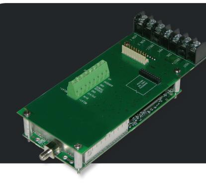
The FGR2 Cathodic Protection remote monitoring radio is a multi-purpose, spread spectrum radio with specific inputs and outputs for monitoring and reporting operational values on pipelines, tanks, structures and other underground facilities subject to environmental corrosion.
